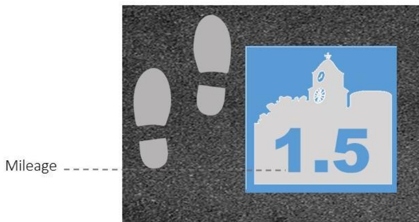
Figure: Prototype Stenciled Pavement Mile Marker
