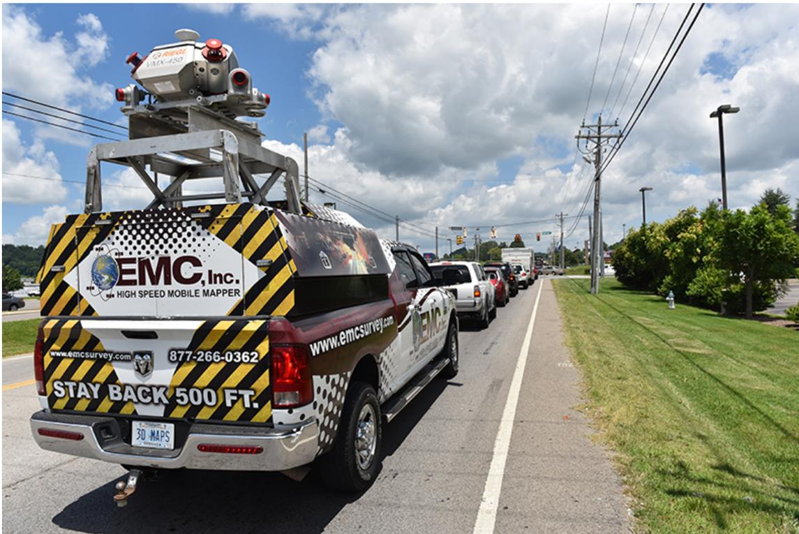
*EMC Inc. collects LiDar mobile mapping data along busy U.S. 31 in Spring Hill on Wednesday, July 15, 2015, that will be used to create a topographical survey map to help determine right-of-way limitations and cost estimates for a potential U.S. 31 widening project.*
